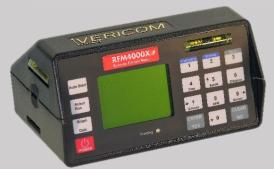
The Vericom VC4000 series Runway Friction Meters are FAA Approved for Airport Winter Safety – as defined in *FAA AC 150/5200-30D; Performance Standards for Decelerometers*. All instrumentation is contained in one easy to use device. With the Vericom VC4000 RFM you are assured of consistent and precise testing between users. The Vericom RFM4000 series reports Mu to support FAA requirements for the Runway Condition Assessment Matrix (RCAM).
